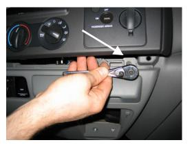
Remove (2) upper hex screws located under the upper portion of the trim.
